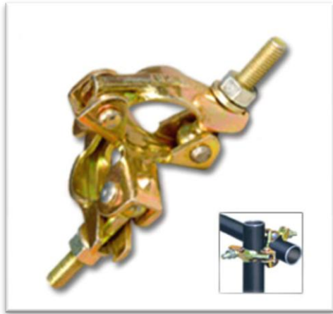
DOUBLE COUPLER For pipe OD 48.3 mm (EN-74 / BS-1139)
